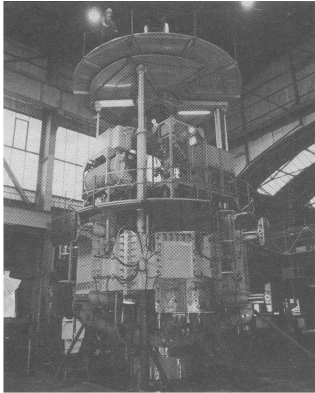
fig. 2: WIRTH down reaming machine type SB VII-650/850
